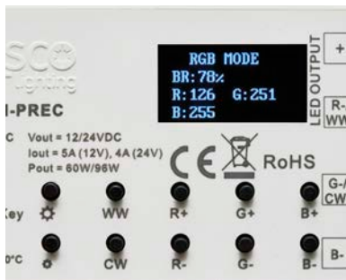
Display in RGB mode. RGB values can be tuned in increments of 1
